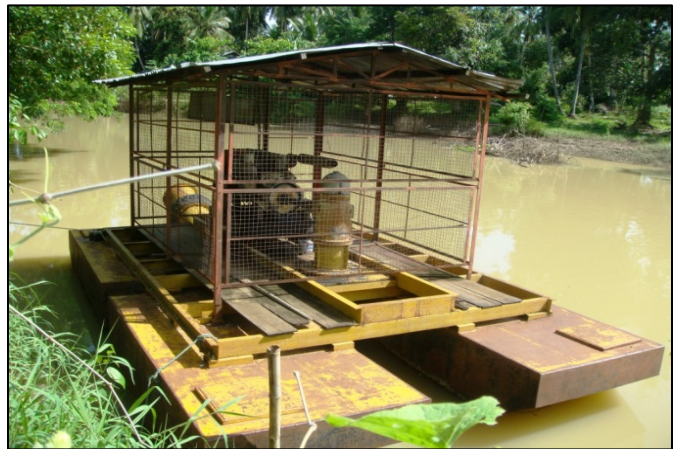
Picture 3 Example of pump and motor on floating pontoon (Cambodia)
