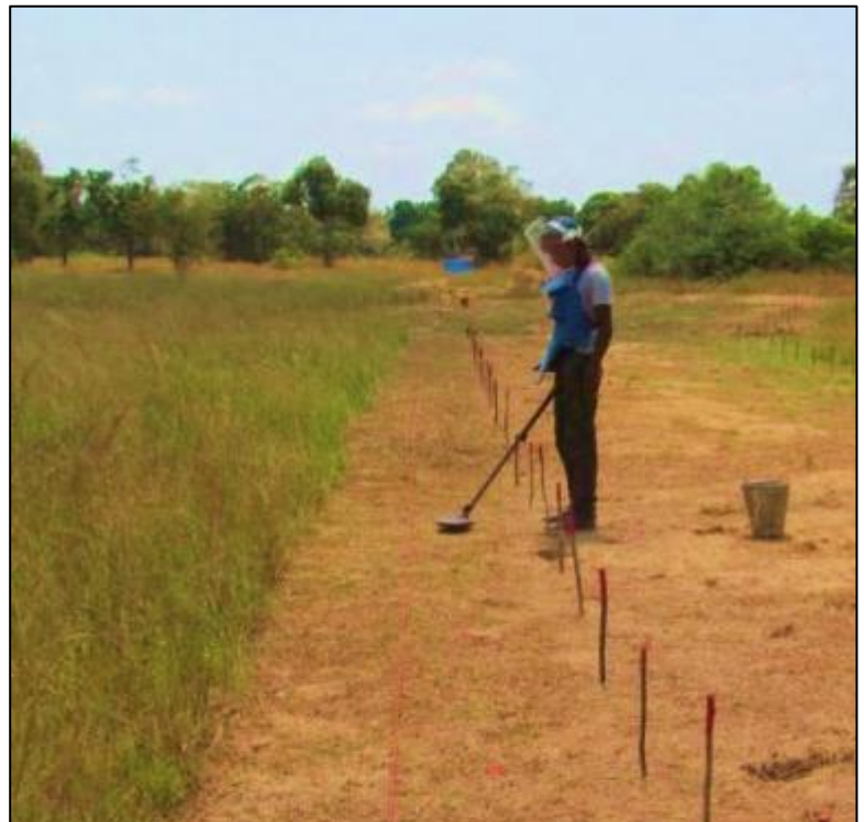
A deminer conducting clearance using the linear method, which allows the deminers to work along long strips of land greatly improving efficiency and fluidity
