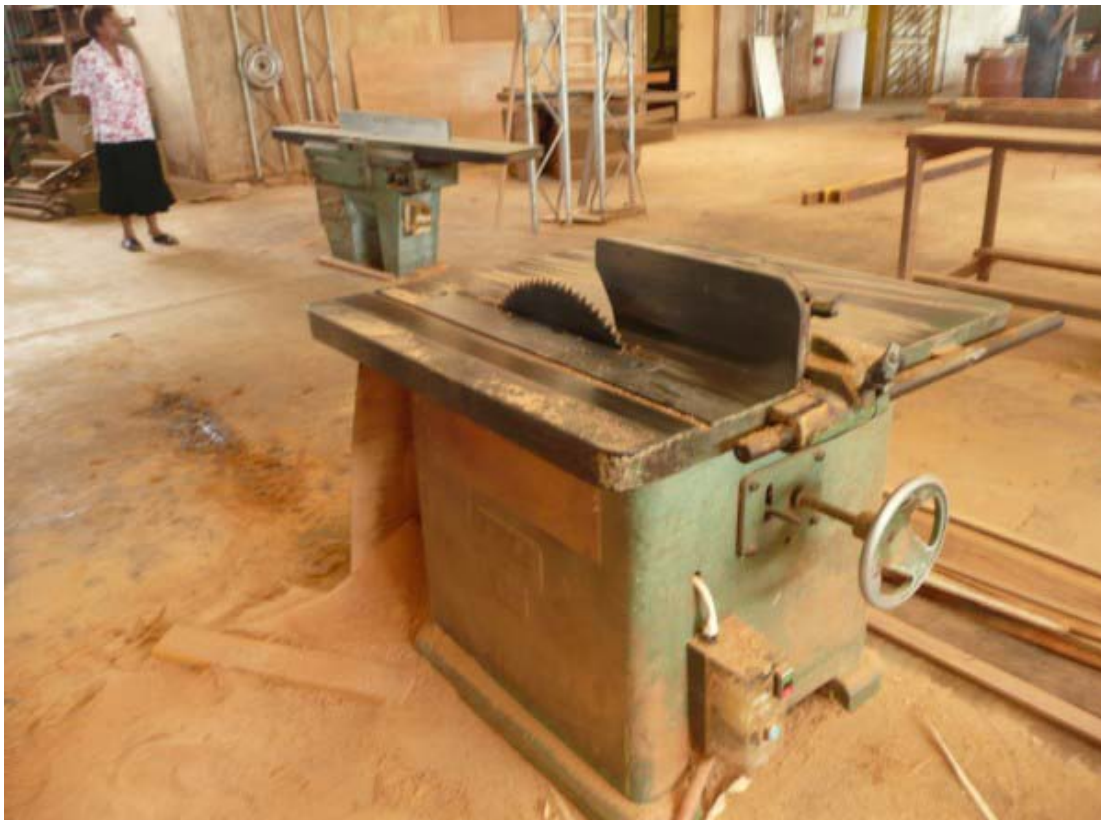
Dangerous rip saw bench. No guards, riving knife or extraction system
