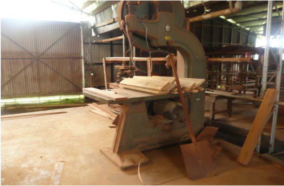
Large band saw no longer operable, needs replacing
