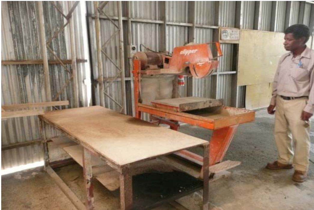
Masonry saw no longer operable
