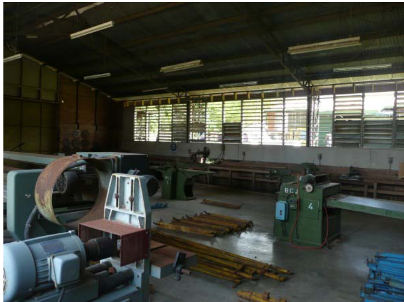
Carpentry machinery many no longer working and no extraction system connected.
