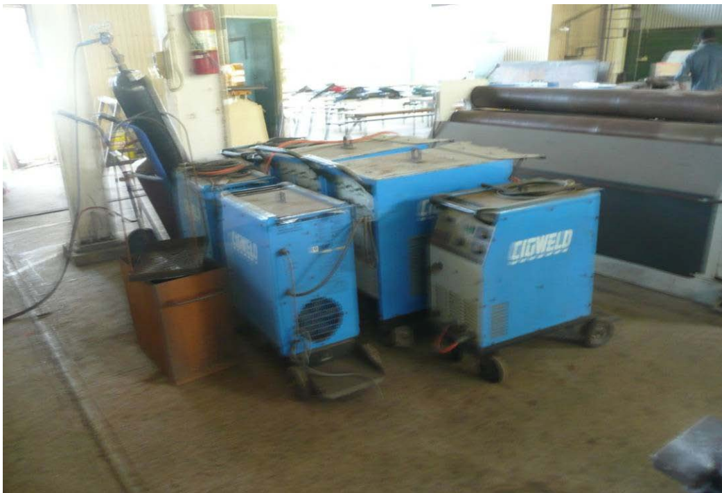
TIG and MIG welding machines no longer operable
