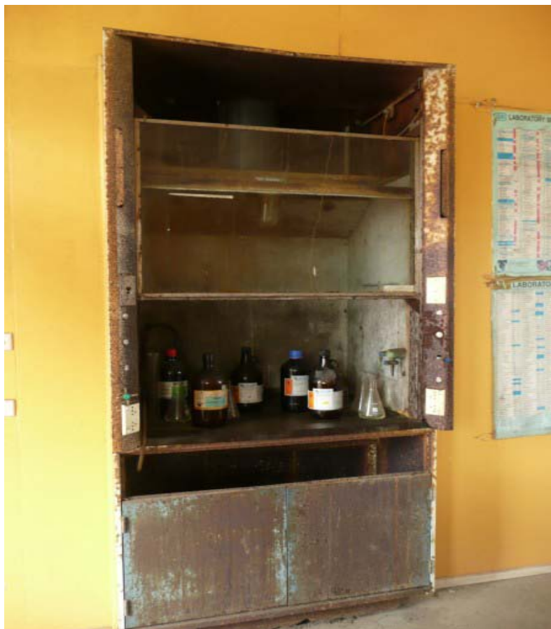
Severely corroded fume cabinet, not working
