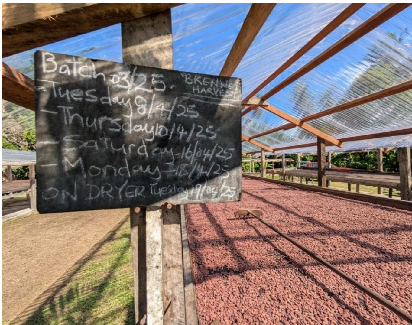
Figure 2. A solar dryer in action used for drying cocoa, batch dates are handwritten on the blackboard (PHAMA Plus)
