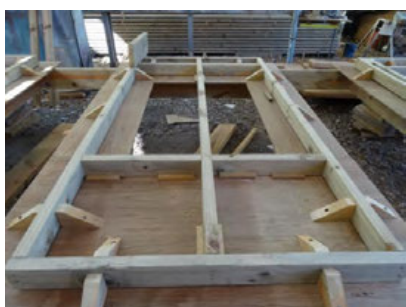
Kitset window module under fabrication at the Kitset Factory
