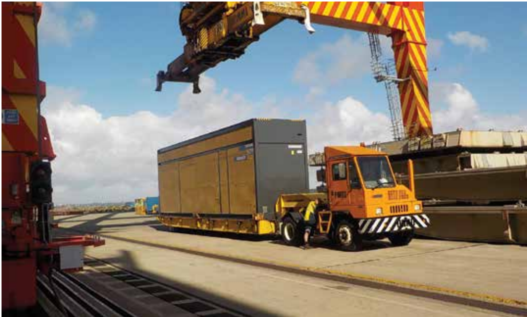
Our first prefabricated chancery—for our post in Rabat—was built, tested and commissioned in Sydney in collaboration with the Australian prefabrication construction industry. It was loaded at Port Botany for shipping to Morocco [C.C. Pines/ Admiralty Maritime Consultants]
