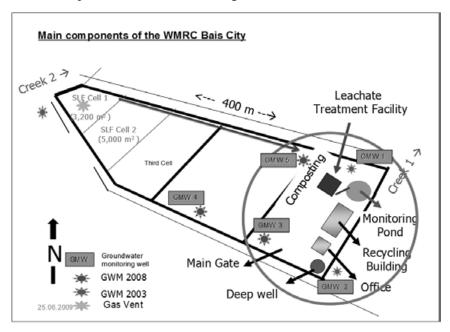
The following sketch shows the measurement grid but also indicates the areas and time of waste disposal at the various monitoring points and filled landfill units.
