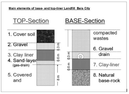
To apply the concept at the Bais City landfill, several changes were proposed for the top cover arrangement, as seen in the diagram.
