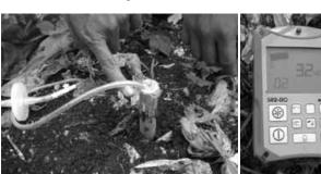
At every monitoring point, the gas detector was used to measure O2, CO2 and CH4 concentrations at the surface and at a depth of 0.5–0.6 meter below surface.
