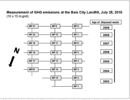
The following graph shows the first landfill unit of around 0.5 hectare that was filled from 2003 to 2009.
