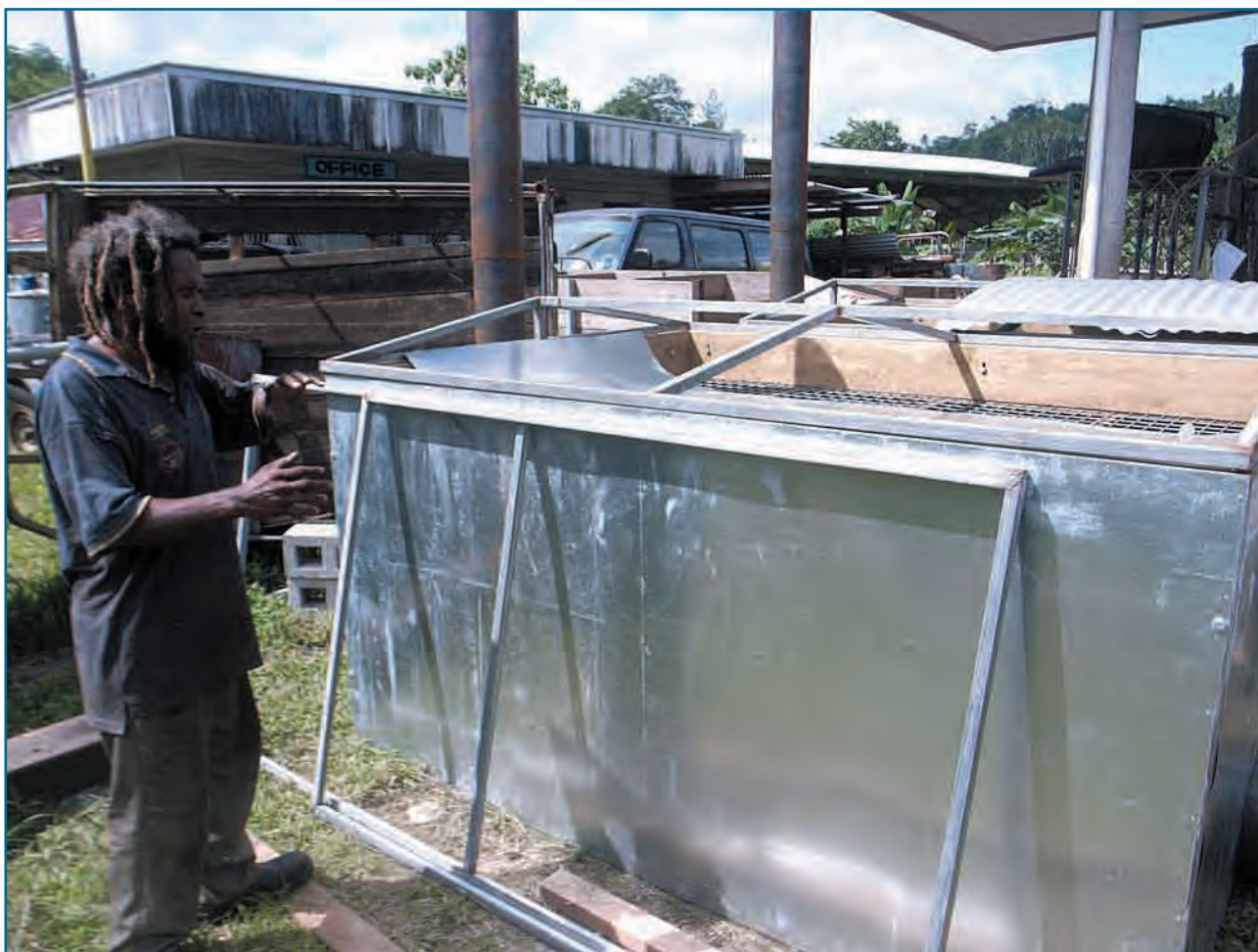
Fabrication of mini driers for CLIP by welding enterprise in Auki, Malaita
