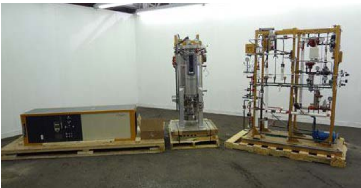
Figure 2.E. A 1000-litre fermenter packed for transit together with its control unit (left) and steam generation apparatus (right).
