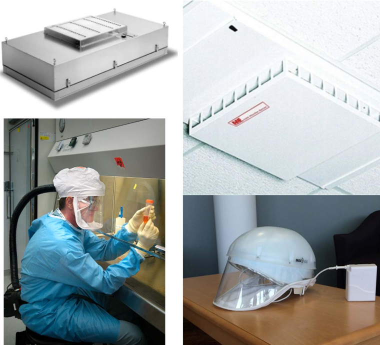
Figure ARG 3.A. Self-contained, fan-HEPA filter units. Top left: a unit with an air inlet visible and the HEPA filter hidden from view. Note the clamps to secure the HEPA filter to the fan unit and the hooks for hanging the unit from the ceiling. Top right: the HEPA outlet side of a similar unit installed in a ceiling. Bottom: battery-powered personal fan-HEPA filter units can be worn during work in P3/L3/BL3/BSL3 containment facilities. In this unit, the fan and HEPA filter are small. Filtered air is blown into the clear facemask.
