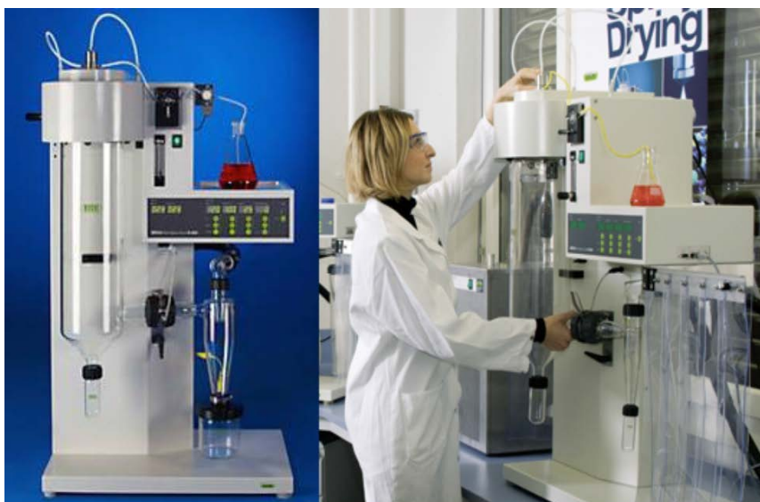
Figure 6.B. Controlled spray dryers. These spray dryers have water evaporation capacities of \sim 1 kg/hr.
