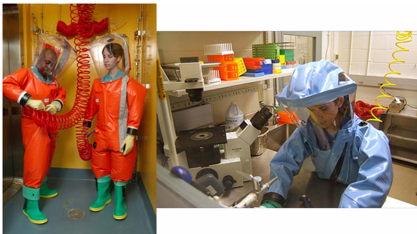
Figure 7.A. Examples of full suits with tethered air supplies. See also Figure 1.B for a picture of personnel in full suits.
