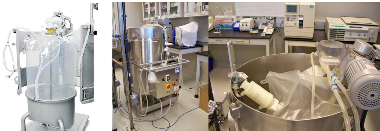
Figure 2.D. Stirred tank reactor-type disposable fermenters. Left: A stirred tank reactor with the cultivation chamber inflated. Right: A different cultivation chamber holding device with the cultivation chamber deflated.
