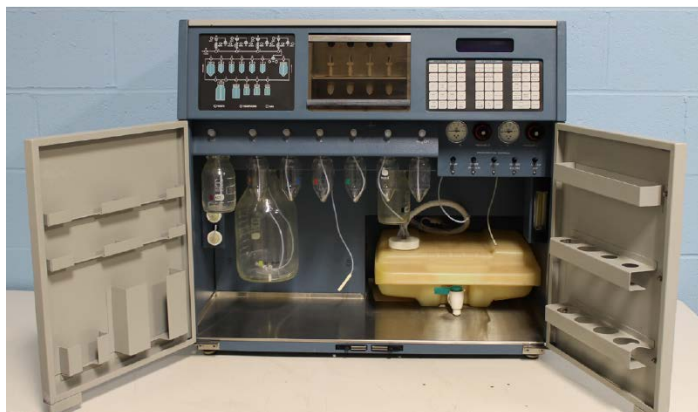
Figure 10.D. A used DNA synthesizer. This equipment is capable of DNA synthesis only (not assembly). It cannot produce continuous nucleic acids longer than 200 bases (0.2 kilobases).
