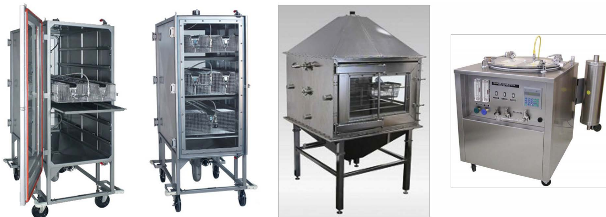
Figure 8.A. Whole-body aerosol inhalation chambers with integral containment systems. Note the connections for sensors and sampling on the side of the chamber in the second photograph from the right. The chamber on the far right contains a basket that can hold multiple mice for whole-body exposure.
