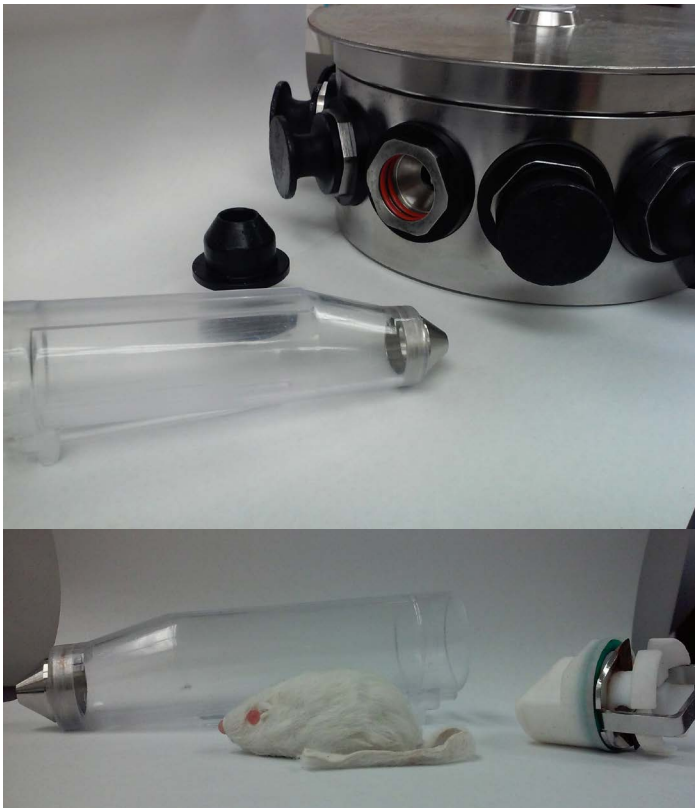
Figure 8.D. Close up views of one tier of a stackable central plenum and closed rodent restraint tubes. Note the polished metal used to construct the plenum as well as the multiple O-ring
