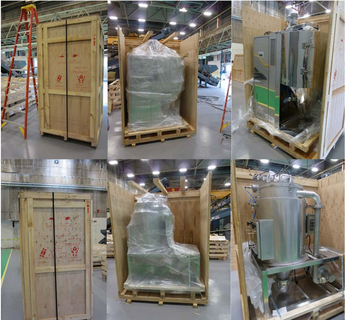
Figure 6.D. Spray dryer removed from shipping crate and shrink wrap following delivery. Top three images: the drying chamber, heater, and control unit. Bottom three images: the fine particulate system. This shipment also featured a third crate containing 8–10 cardboard boxes of parts.
