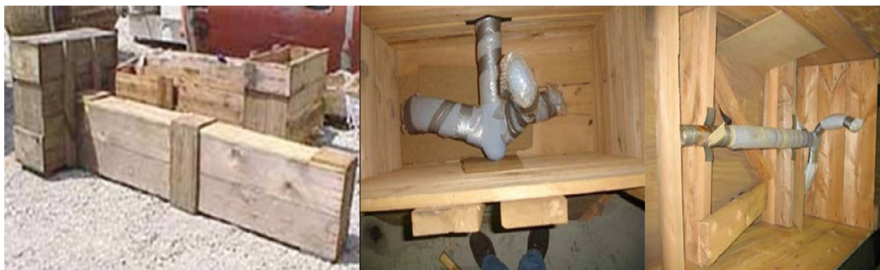
Figure 1.2.F. Crated agitator shaft-impeller units. Left: crate with larger box to accommodate impeller. Centre: protectively wrapped glass -lined impeller. Right: view of wrapped and shaft in a simple rectangular crate.
