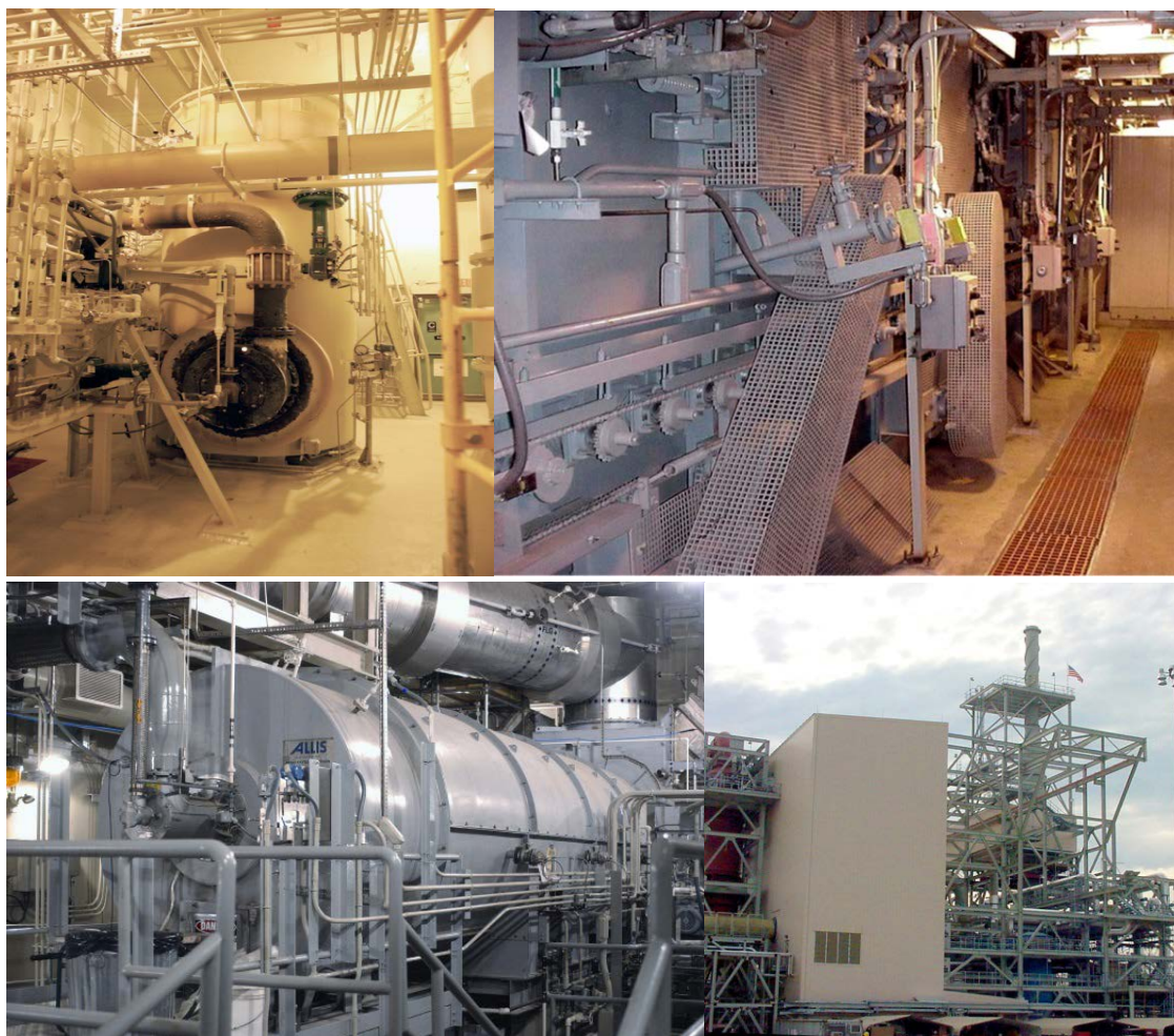
Figure 9.B. Facilities for chemical agent incineration operations. Top left: liquid incinerator. Top right: metal parts furnace. Bottom left: deactivation furnace. Bottom right: pollution abatement system.
