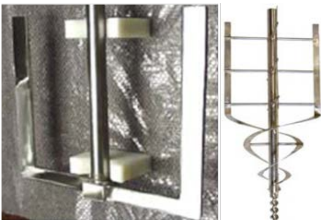
Figure 1.2.C. Agitators for high-viscosity applications. Left: anchor type. Right: hybrid helix anchor design.
