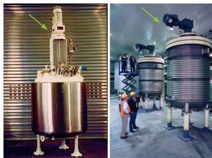
Figure 1.1.B. Chemical reaction vessel designs with agitators. The green arrows point to the agitator motors protruding from the tops of the vessels. Left: 500-litre glass-lined reactor with welded top head and smooth sides. Right: Reactors with visible temperature control coils and bolted top heads.
