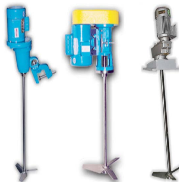
Figure 1.2.A. Complete agitators with a variety of motor and mounting options. Left: Gear drive motor with C-clamp mount. Centre: Belt drive motor with flanged mount. Right: Gear drive motor with angle riser and plate mount.
