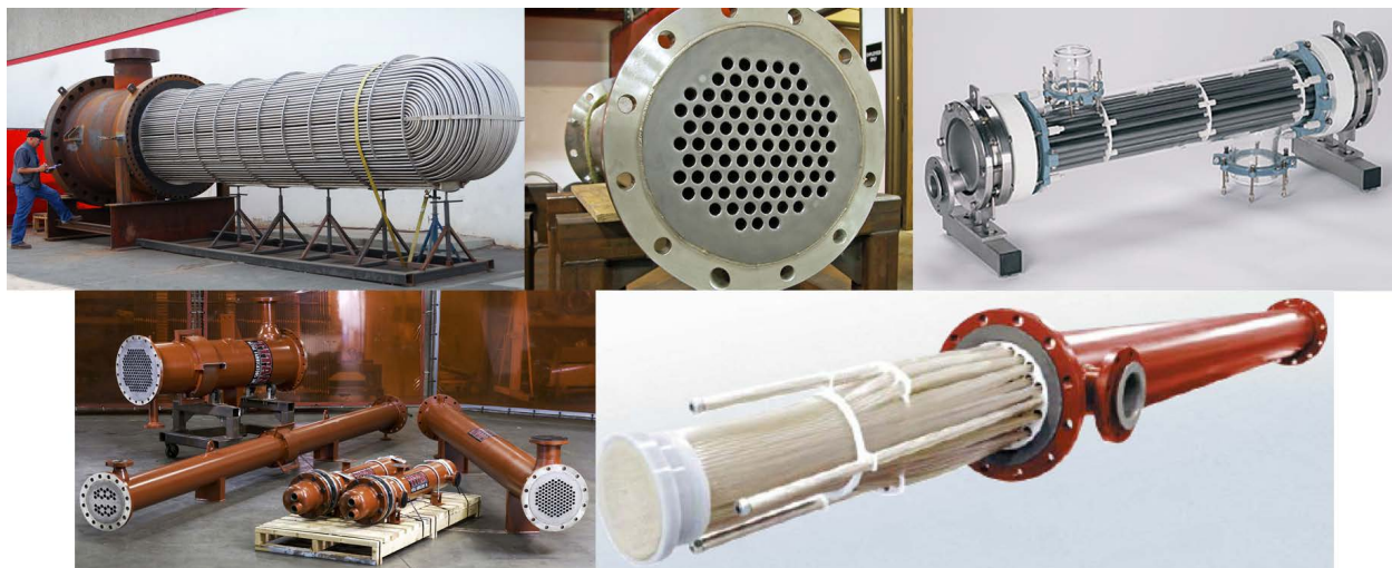
Figure 3.B. Shell and tube heat exchangers. Top left: U-shaped tube bundle made from high-nickel Alloy 625 . Top centre: end view of a tantalum tube sheet. Top right: heat exchanger with silicon carbide tube bundle and glass shell. Bottom left: tantalum heat exchangers with a variety of sizes, tube arrays, and fluid connections; note the heads with fluid connections on the palletted heat exchangers. Bottom right: heat exchanger with fluoropolymer tube bundle pulled out.
