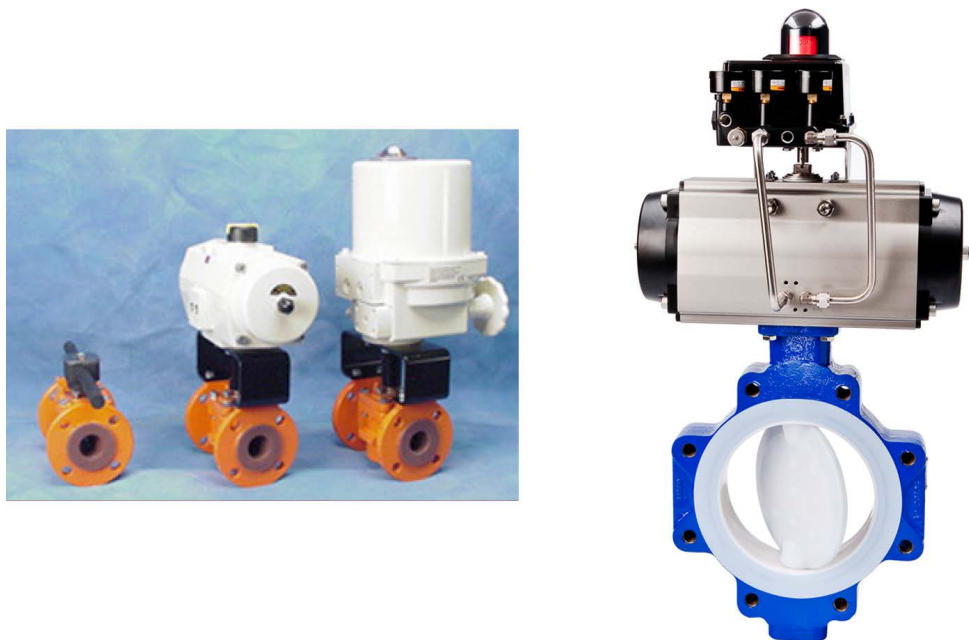
Figure 6.A. Fluoropolymer valves in a variety of designs. Left: PFA-lined plug valves with different actuation mechanisms (manual, pneumatic, and electrical). Right: DN150 PFA-lined butterfly valve with pneumatic actuator, indicator, and limit switch enclosure.
