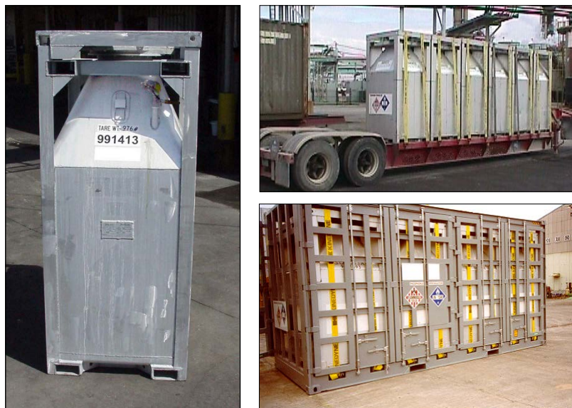
Figure 47.B. Aluminium tote bins used for shipping bulk quantities of phosphorus pentasulphide. The single bin on the left measures 218 cm × 112 cm × 132 cm and holds up to 2636 kilograms of the solid. The top right photograph shows a low-boy trailer hauling six tote bins, and the bottom right photograph shows a cage container for tote bins.
