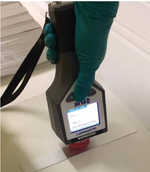
IAEA measurement of uranium in target plates used for radiopharmaceutical production using an HM–5 detector (Credit: ANSTO).
