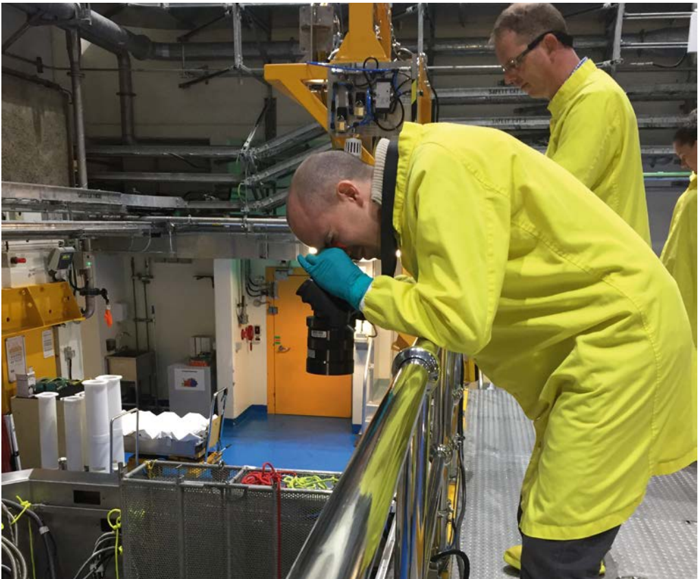
ANSTO inspection – IAEA inspector using ICVD Cerenkov Device and Stephan Bayer (ASNO) (Credit: ANSTO).
