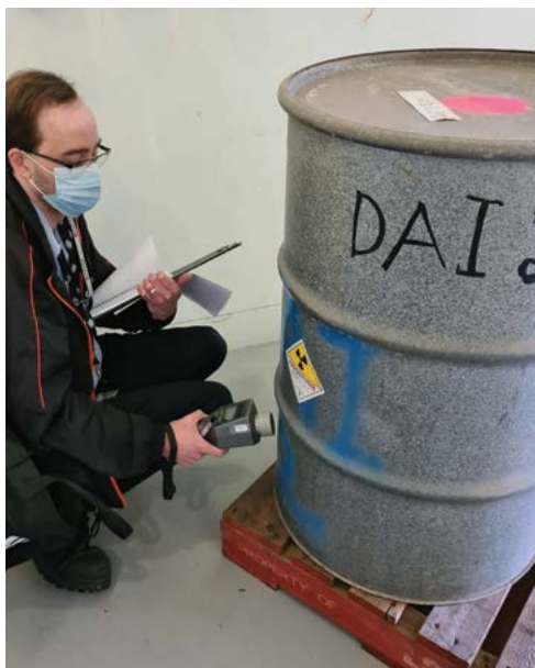
ASNO inspector performing a measurement with an HM-5 handheld spectrometer during IAEA Complementary Access at CSIRO, 28 August 2020.
