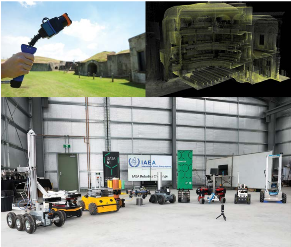
Top left: The “Zebedee” – a hand-held 3D laser mapping device developed by CSIRO, which the IAEA uses in nuclear safeguards inspections. Top right: A “Zebedee” map of the Opéra-Théâtre de Clermont-Ferrand, used to demonstrate the potential applications of the device. Bottom: In 2017 ASNO brought the IAEA and CSIRO together to conduct the Robotic Challenge, where teams tested their robots’ abilities to assist IAEA inspectors in performing safeguards tasks.
