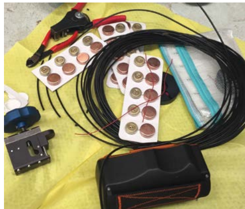
IAEA seals and sealing tools used for dual containment and surveillance during the inspection with the AWCC, August 2020.
