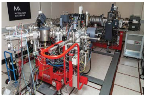
Large-geometry secondary ion mass spectrometer (LG-SIMS) at University of Western Australia's Centre for Microscopy, Characterisation and Analysis. (Credit: UWA)
