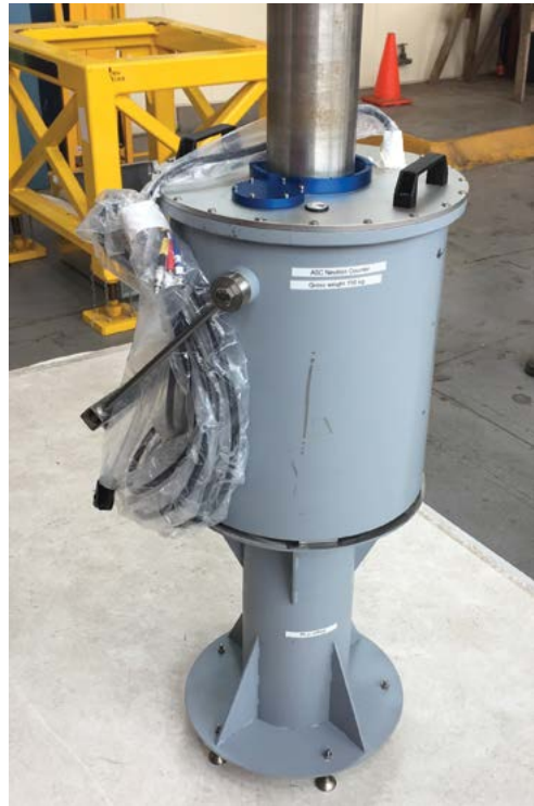
The active well coincidence counter (AWCC) used during the interim inventory verification inspection at ANSTO in August 2020.
