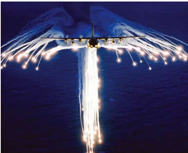
A Lockheed C-130 aircraft deploys infra-red flares in order to decoy heat-seeking missiles away from the aircraft. (Photo: US Air Force)
