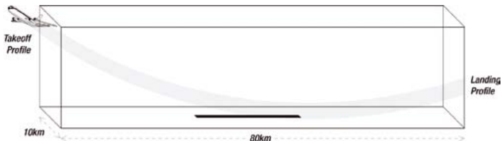
Figure 2. The typical area around an airport runway where an aircraft might be in danger from a ground-launched MANPADS missile. The total area is around 800 square kilometres.
