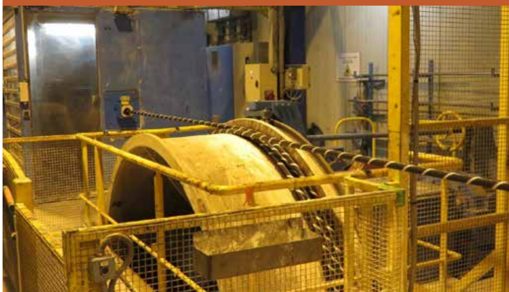
The Coral Sea Cable on the cable armouring line at Alcatel Submarine Networks. Photo: Vocus Communications
