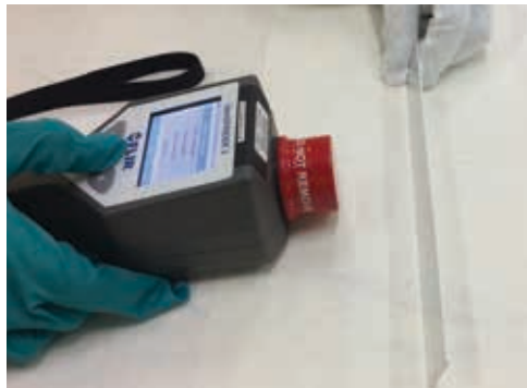
IAEA inspectors performing a measurement on a target plate used for molybdenum-99 production at ANSTO during physical inventory verification in May 2019.
