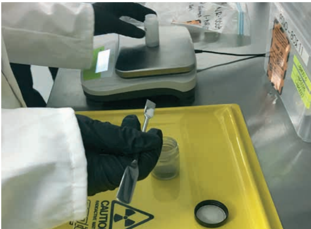
Taking a sample of nuclear material for analysis during physical inventory verification at CSIRO – Black Mountain in May 2019.
