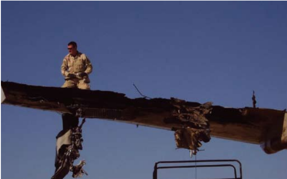
Damage caused by a fire in the wing of an Airbus A300 struck by an SA-14 MANPADS missile on departure from Baghdad airport in November 2003. (Photo: US Department of Defense)
